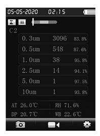
8. Press "deactivate" in the "filter efficiency" menu to switch the filter efficiency mode back off again.
